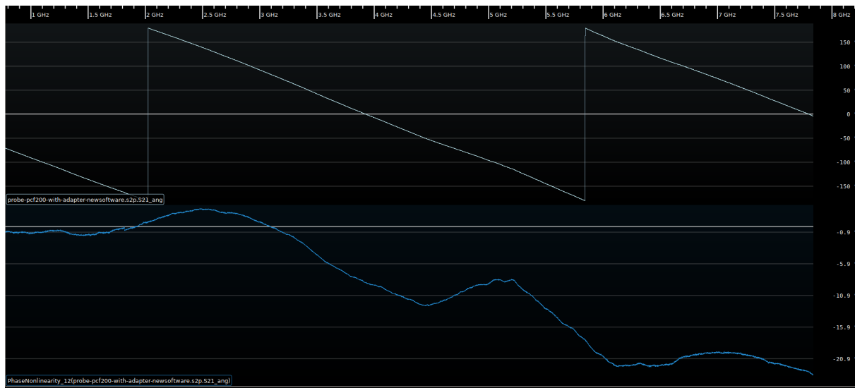
Figure 15.15: Example of nonlinear phase of a filter in the stopband
